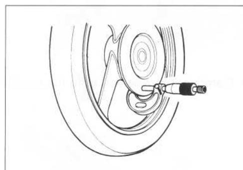
Measure the runout with a dial gauge.
