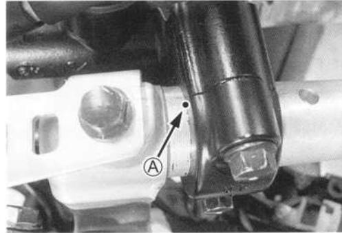
**🔧 Front brake master cylinder mounting bolt: 10 N·m
